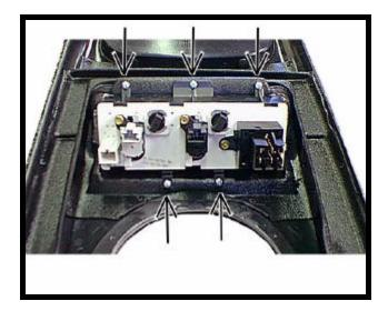
5. Remove two (2) plastic tabs on secondary light and pod assembly, replace two (2) OEM screws in front assembly as shown. See Figure 12.
